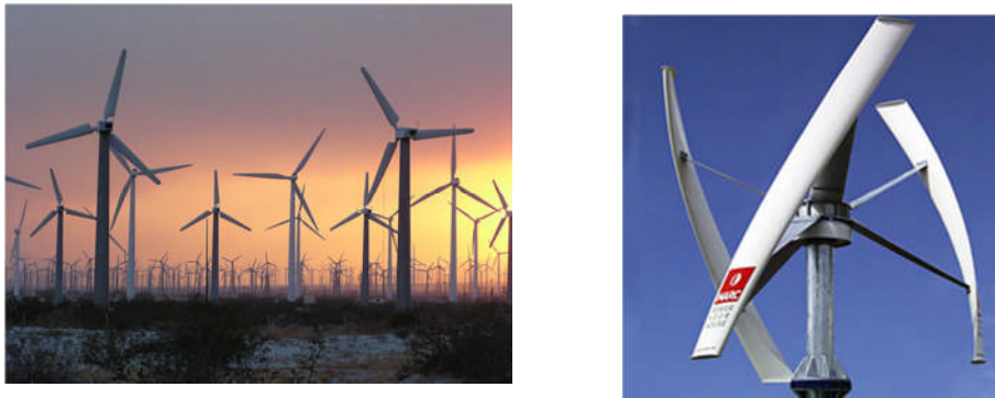
Figure 17: "Modern" horizontal axis (HAWT) and vertical axis (VAWT) designs [9]
