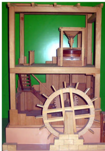
Figure 2: Reconstruction of Vitruvius' undershot-wheeled watermill
